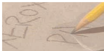
An electronically charged pencil rotates the bichromal beads in a sheet of Xerox electronic reusable paper.
